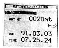
When **ENT** is pressed following the UTC date and time entry, the display resets to the normal "Auto Start up Sequence".
