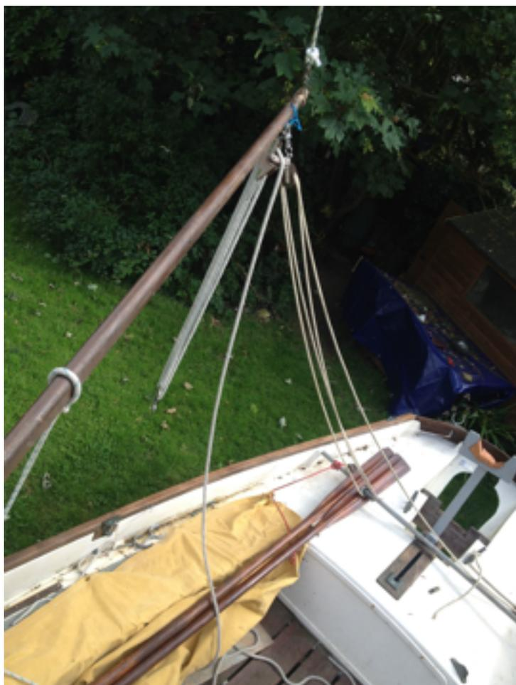
Now for testing; we put axle stands under the rear of the trailer and wood blocks under the end of the boats keel plank, to stop her tilting back, then attached a large bucket of water to the hoist to test its steadiness. We were a little concerned that the whole boat and trailer would tilt\*\*, but it didn't and allowed us to more easily lift the engine up and over the gunwales and then be swung across midships.
