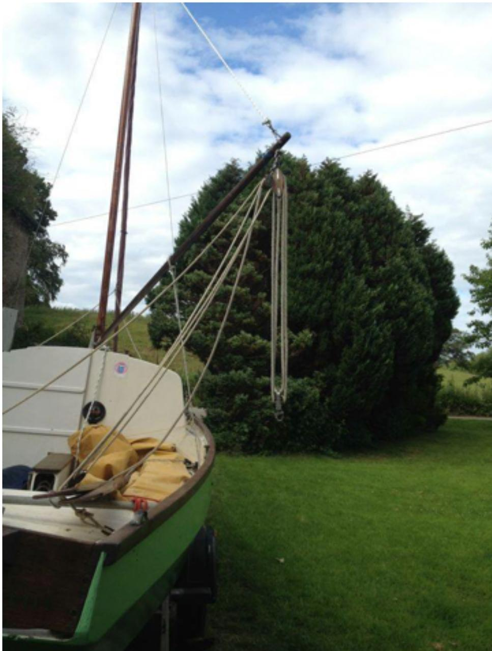
We set up the main halyard as the principle way to hold the boom in place and to be able to raise and lower it. I had taken off the boom anyway as I intend sailing her loose footed for now.
