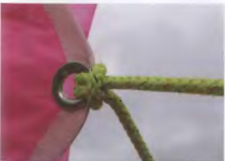
Larks foot the sheet to an asymmetric spinnaker
