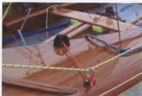
Twinning lines provide greater control
