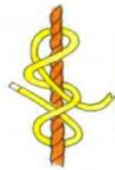
Rolling hitch Used when you need a knot that won't slip when pulled at an angle. Ideal for taking the strain off another rope.
