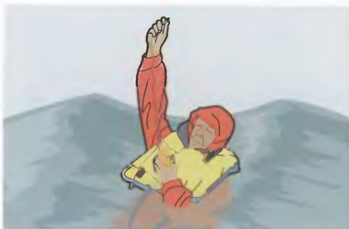
The MOB should hold the antenna as high as possible to give the greatest range.
