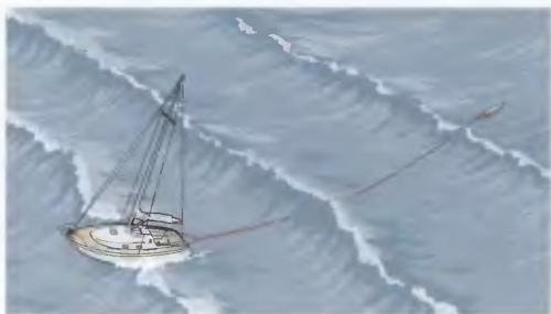
Drogues help prevent broaching and twisting sideways onto the waves.
